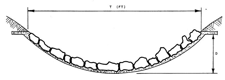
MINIMUM 4" CONCRETE OR GUNITE GROUT, WITH NATIVE BOULDER RIP-RAPP EMBEDMENT, 6x6-6/6#W.W.MESH MINIMUM REINFORCEMENT. (0.5T)<sup>2</sup> = C(D) WHERE C = PARABOLIC CONSTANT
