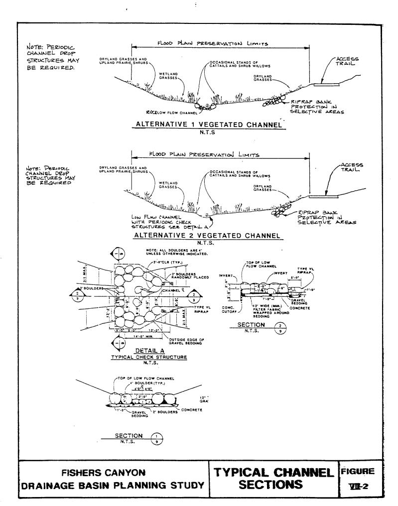
Fishers Canyon Drainageway and Tributary: Alternative 2 - Vegetated Channel with Periodic Check Structures. This concept is similar to Alternative 1 but proposes the use of small periodic check structures instead of a continuous rock low flow channel. Between check structures the low flow channel would be unlined and would be allowed to erode and flatten over time to a stable equilibrium slope. Additional information comparing Alternative 2 to Alternative 1 is shown in Table VII-3.
