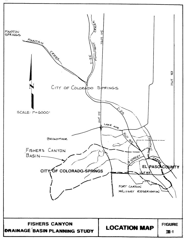
in El Paso County, tributary areas slope toward the central drainageway at two to five percent. The elevation of Fountain Creek the eastern limit of the basin is 5,720 to 5,770 feet above sea level.
