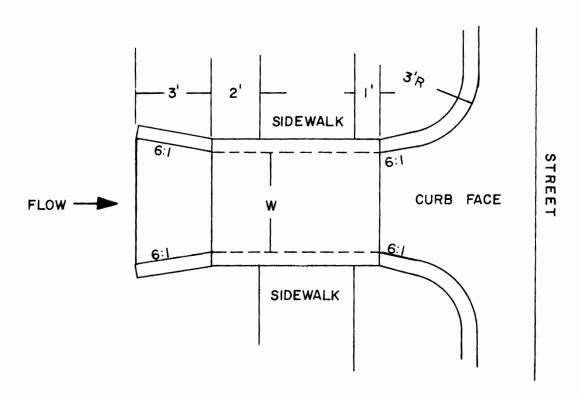
6" CONCRETE WITH NO.4 BARS AT 12" CC IN BOTH DIRECTIONS
