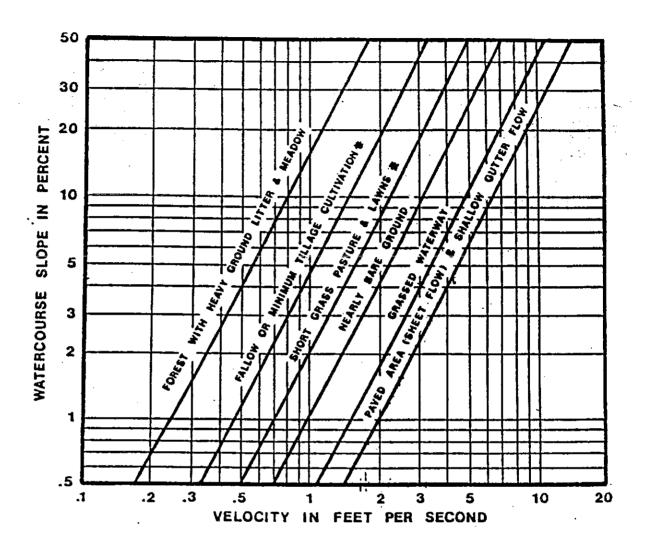
FIGURE 3-2. ESTIMATE OF AVERAGE FLOW VELOCITY FOR USE WITH THE RATIONAL FORMULA.
